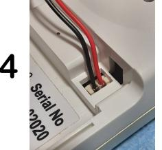
Continue pushing down until you hear the plug click into place; the machine will also "beep" when it's fully inserted
