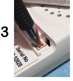
Using something small and pointed (ex. pen, pencil, small screwdriver), push the 4 corners of the plug into the port
