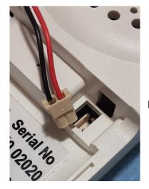
Insert battery plug into the machine's port
