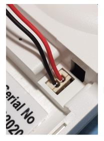
Initial placement – this is NOT fully inserted into the port
