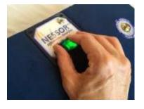
NOTE: To extend the life of the batteries make sure that the Nessor is turned off at the end of the session. The Nessor is off when the green button is in the middle position.
