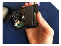
**Step 3**: The batteries are in the rectangular black box. Slide the lid out and remove the 2 triple A batteries.
